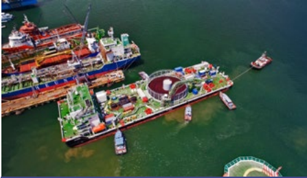
Conversions of Flat Top Barge to Cable Laying Barge
